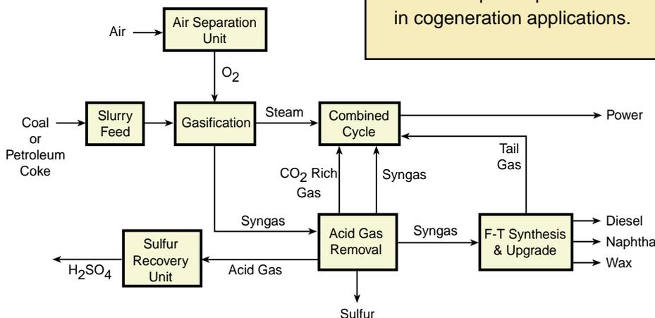
Texaco Energy Systems process flow diagram
