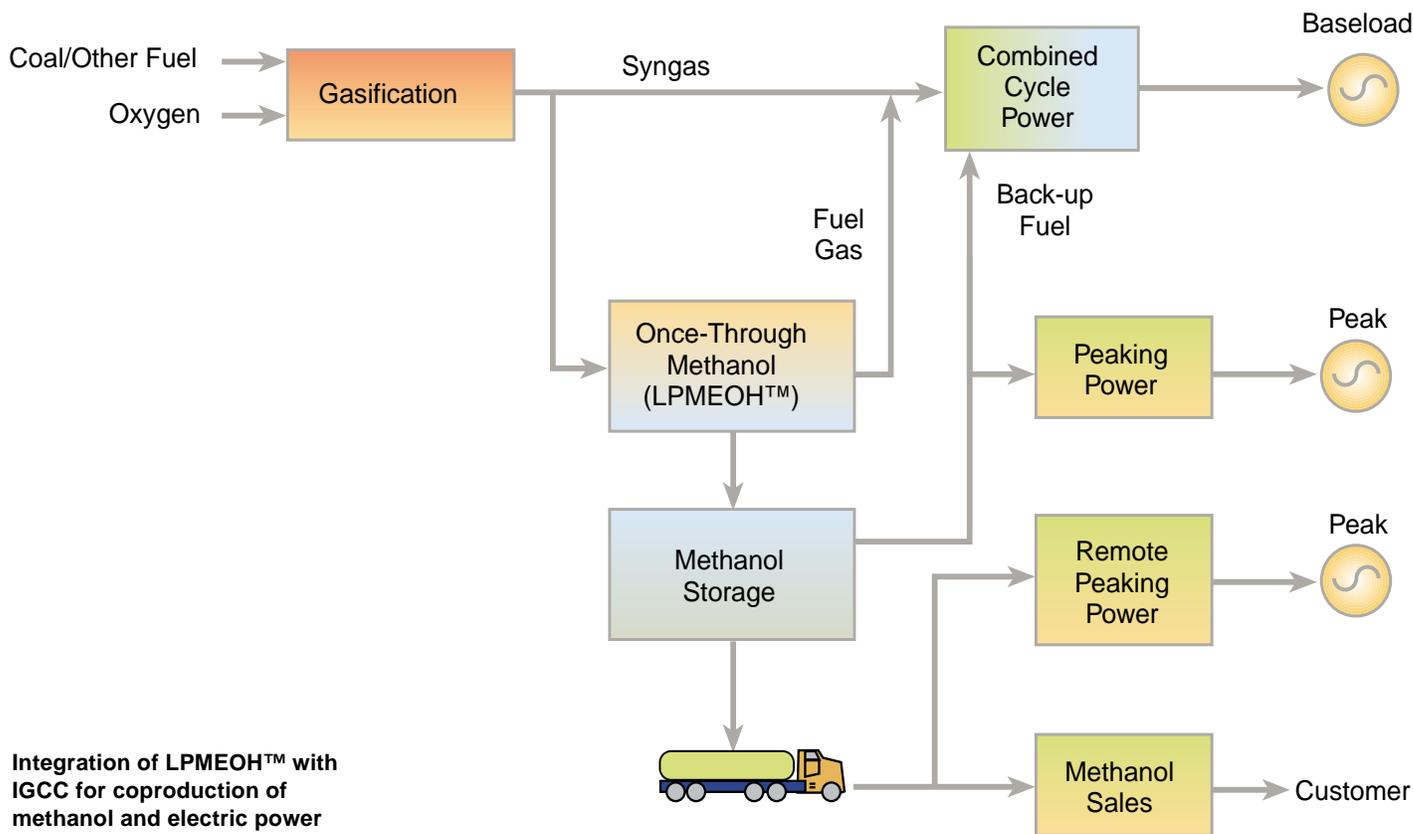
Integration of LPMEOH™ with IGCC for coproduction of methanol and electric power
